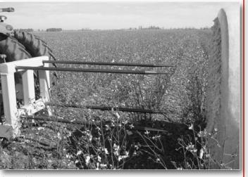
module, slowly back up until the modules touch, pull forward 4-8 inches, drop the hitch all the way down and pull away. There is no resistance on the cotton spears when the tractor pulls away. The module does not roll as much with the Cotton Spear as with other handlers so there will be less time spent keeping the modules straight for truck pick up.
